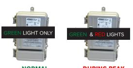
NORMAL DURING PEAK IF BREAKER IS TURNED OFF, RCS WILL GO THROUGH A 10-MINUTE START SEQUENCE WHERE LIGHTS ALTERNATE ON/OFF
