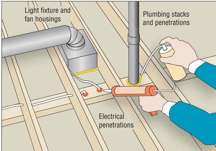
Any item that pokes through the building envelope is a candidate for sealing. Use caulk and spray foam for most applications.
