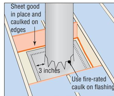
the ceiling in the living space or foundation area, a metal flue pipe will be incorporated. This flue should always be vented with a positive slope of at least ¼" per foot, be routed upward and out through the roof and never terminate inside the vented attic.
