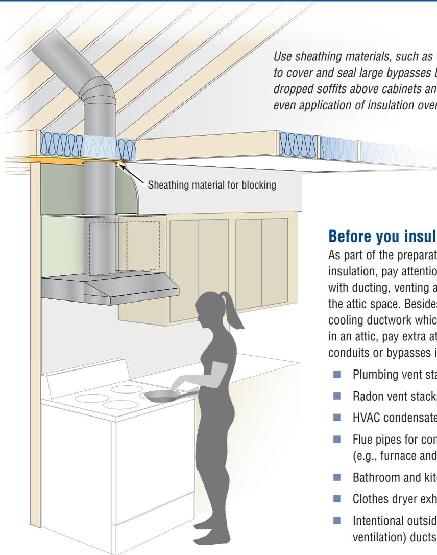
Use sheathing materials, such as OSB board or rigid foam board, to cover and seal large bypasses between dead spaces, such as dropped soffits above cabinets and the attic. This allows for an even application of insulation over those areas.
