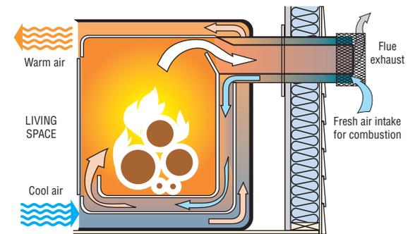
A sealed combustion fireplace provides fresh air for combustion. A heat-exchanging chamber around the firebox improves the efficiency.
